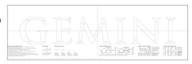
**DRILL PATTERN** (for all other stud mounted products) Computer-generated tracing of letters with hand punched hole locations of studs, printed on 60# white grid paper. Once taped to wall, hole locations are then drilled and filled with adhesive.
