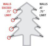
0.25" Standard Wall Thickness **0.75"** Maximum Wall Thickness
